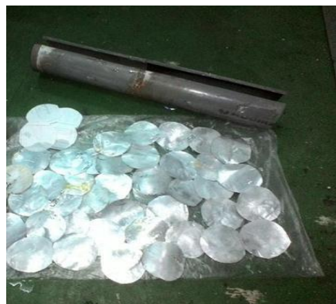
Fig. 2. Preparation of Battery Anod
